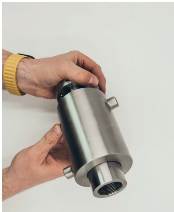
Step 4 - Slide jacket over the vessel body. It is advisable to use O-ring grease, on both the body and O-ring to ensure the O-ring slides effortlessly over the body.
