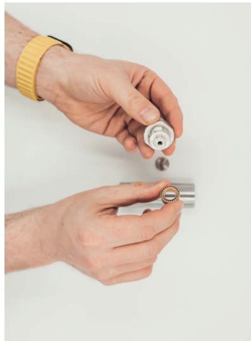
Step 4 - Remove seal
