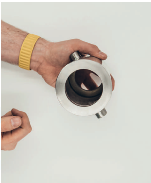
Step 3 - Repeat step 2 and install an O-ring into the lower recess of the liquid jacket.
