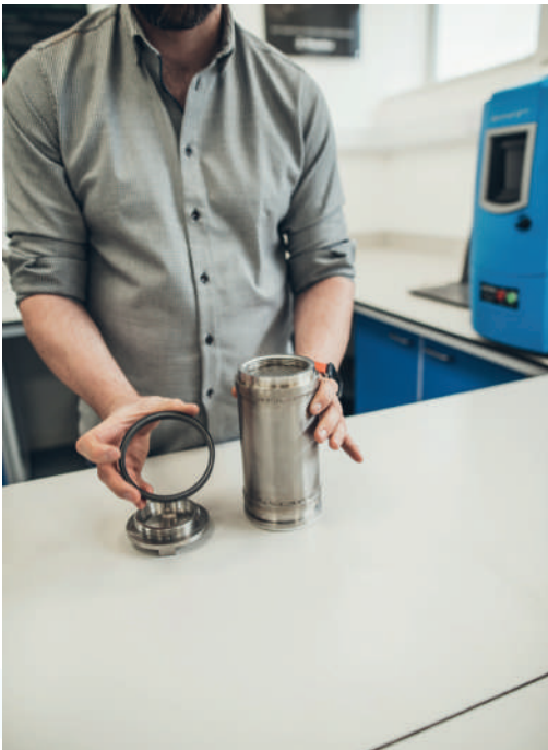
Step 3 - Remove seal
