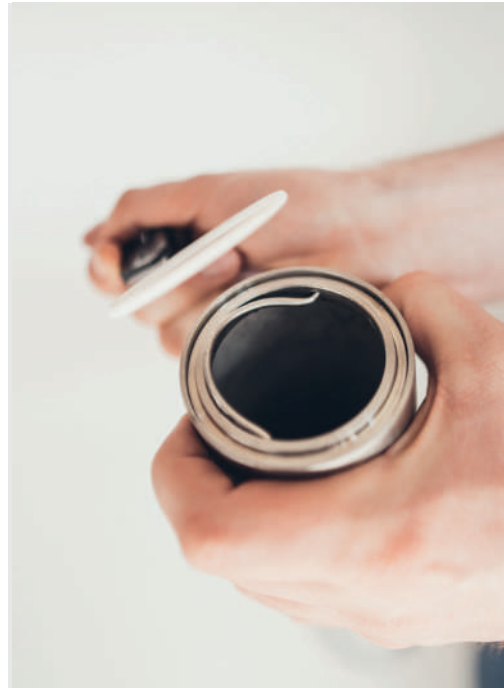
Step 2 - Remove O-ring
