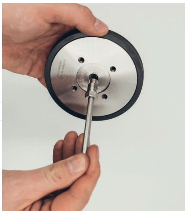
Step 1 - Install the cone and thread fitting as per the manufacturers instructions (autoclave engineer)
