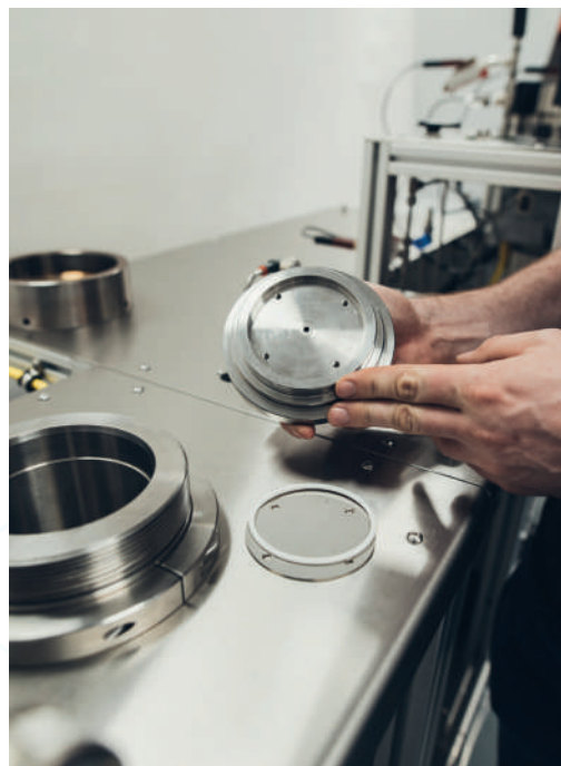
Step 3 - Check PTFE O-ring
