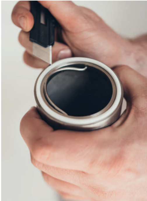
Step 2a - Pierce basket O-rings with a stanley knife or O-ring pick
